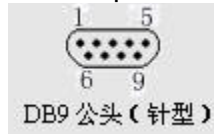
Figure 2. RS232 Pin Definition(Male/Needle Type)
